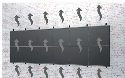
Very good rear ventilation of the modules
